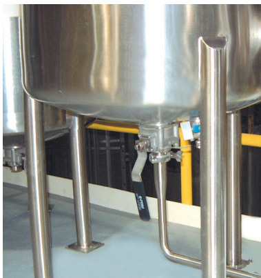
Clean, purge valve in closed position.
